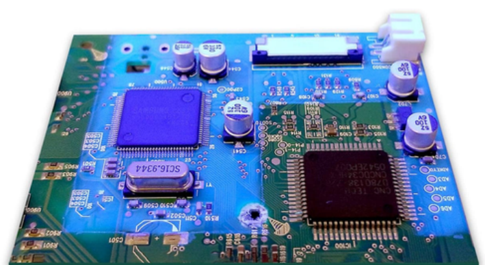
UV inspection of a conformal coated PCB
