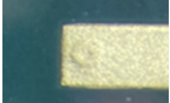
This is a picture of a microvia with a protrusion.
