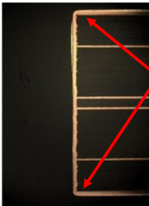
Edge plating wrapping onto outer layer surface.
