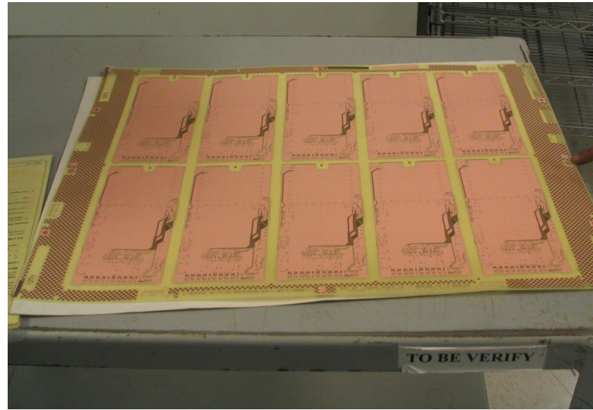
Completed inner layer
